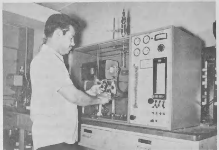
Lab Assistant Mario Croes determines the ppm of sulfur in liquid pentane feed sample using Wickbold combustion procedure.
